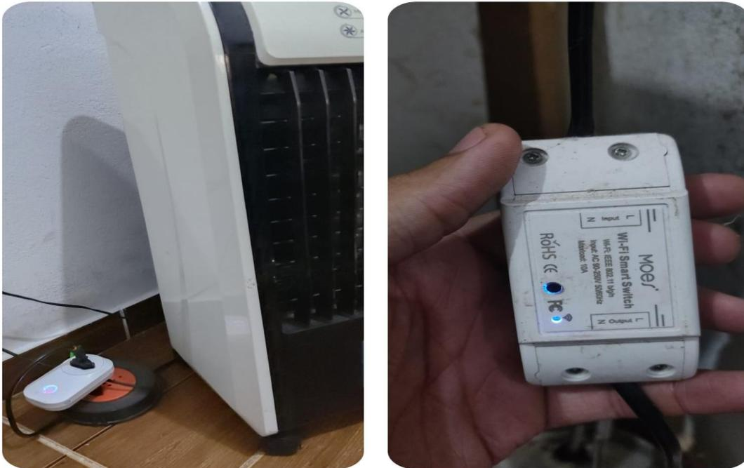
**Figura 29 - Interruptores WiFi (Smart Switch)**
