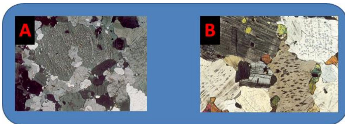
Figure 17 – A) Microperthitic texture in granite. Magnification 34x, XPL B) Antiperthitic texture in tonalitic gneiss. Magnification 20x, XPL. Adapted from MacKenzie et al. (1982).
