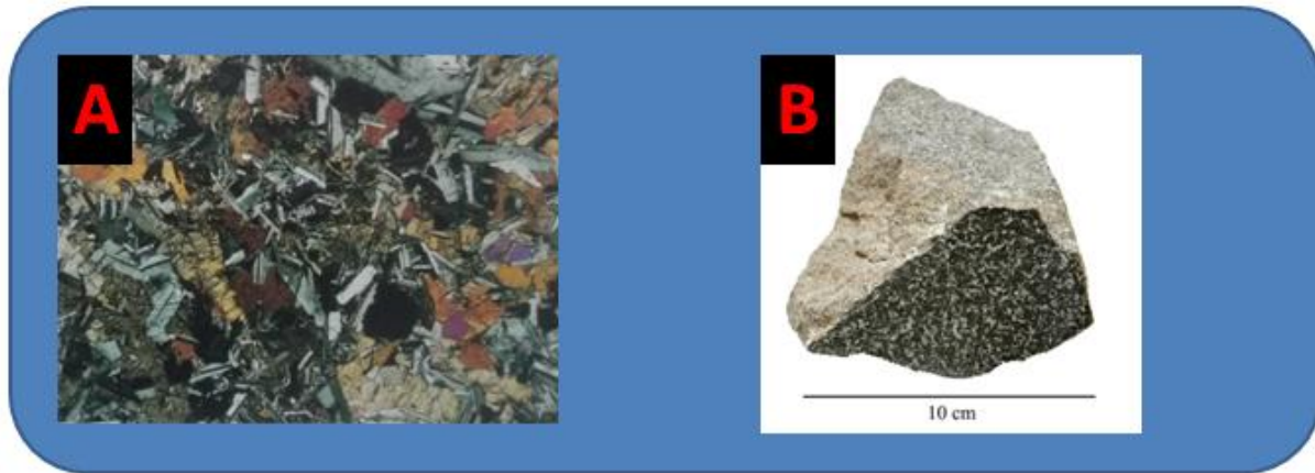
Figure 24 – A) A subophitic tholeiitic diabase, Magnification 21x, XPL. Adapted from MacKenzie et al. (1982). B) Diabase sample. Available in: https://commons.wikimedia.org/wiki/File:Polished_Diabase.jpg
