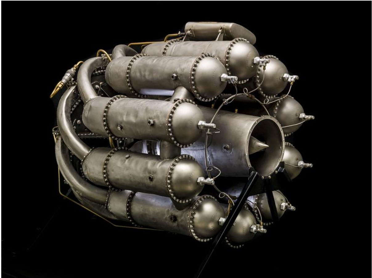
Figura 7 - Motor Whittle W.1X Fonte: National Air and Space Museum (2021)
