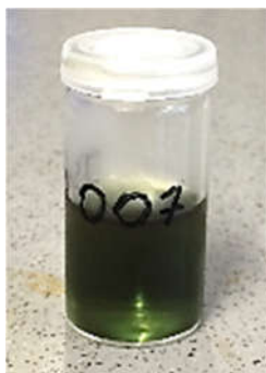
Figure 21: The product suspension after the synthesis of Ag NPs from the experiment VI
