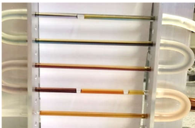
Figure 15: Representation of the flow reactor during experiment III, showing the difference in coloration of the Ag NPs formed during the reaction.
