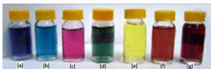
Figure 7: Photograph of (a) Violet (b) Blue (c) Purple (d) Green (e) Yellow (f) Orange and (g) Red Ag NPs suspensions
