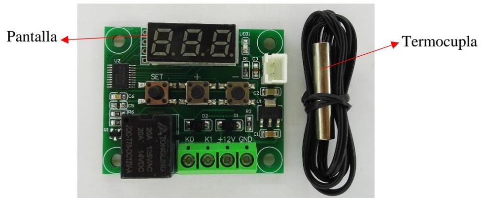
**Figura 5.** Termostato W1209 DC 12V.
