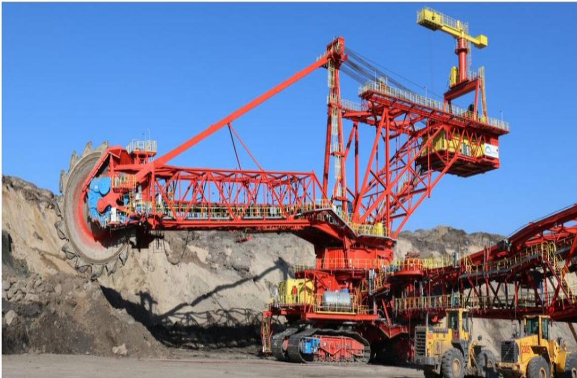
*Figura 9 Bucket Wheel TAKRAF*
