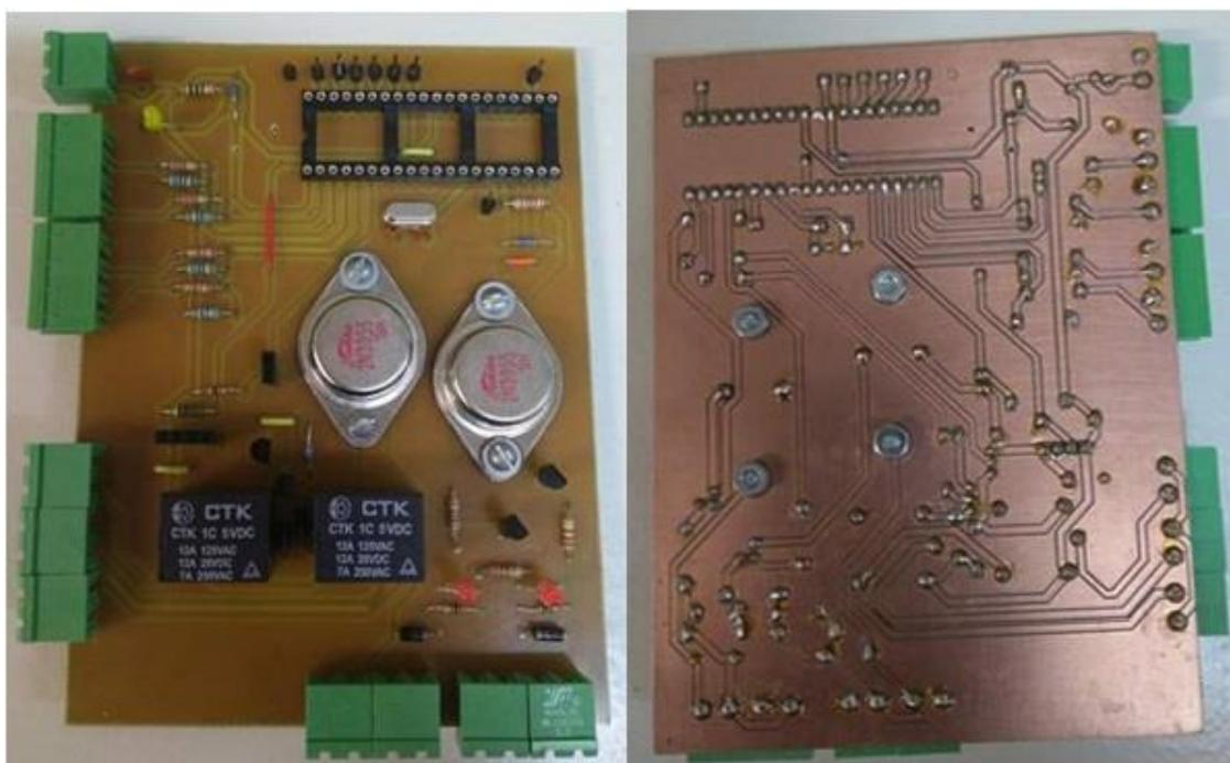
**Figura 44 - Placa de Circuito Impresso do PIC18F4550 (Figuras 27, 28, 29, 30, 31, 32, 33, 34 e 35)**
