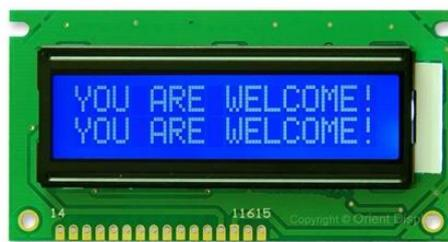
**Figura 2.5: Display LCD 16x2**
