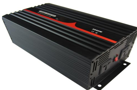
Figura 3.7 – Inversor CTP 3000W off Grid 24V/110V
